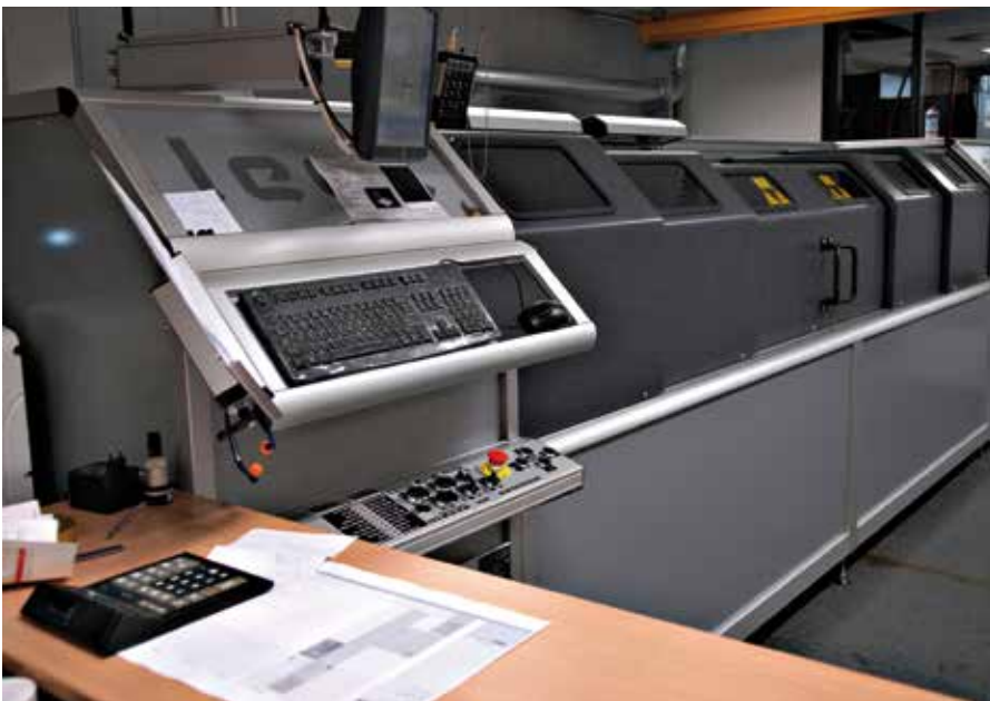
11 Lead CO 2 Laser 'Flexostar Printmaster' graveert flexodrukvormen direct in elastomeer.
